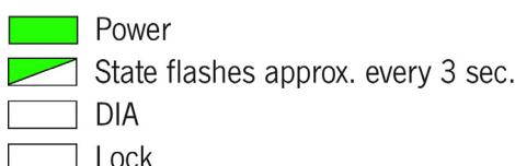
The device displays normal operation with the door open. If this display also occurs with the door close, the handle module has already been taught in and is currently being blocked on this MGB.
